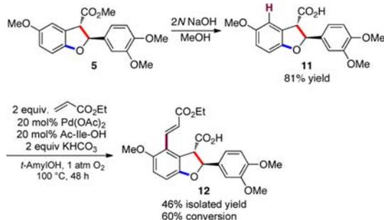
of benzofuranylacrylate **12** in 46% yield (77% based on recovered starting material), which contains key features that are present in the natural product lithospermic acid.<sup>3d</sup> The moderate conversion for the formation of **12** was presumably caused by the highly crowded nature of the flanked C–H bonds.
